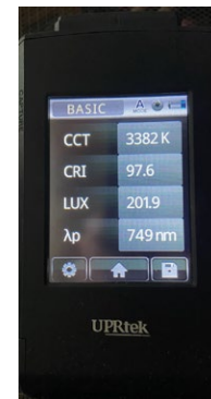
A Light meter with photopic lux and CCT readings
